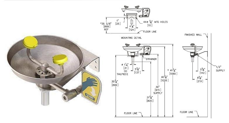
Model S0440-AS is our wall mounted stainless steel eye/face wash complete with stainless steel bowl and mounting bracket. Comes complete with plastic eye/face wash spray heads, an inline strainer and a stay-open 1/2" ball valve with a push handle. Compliant to ANSI Z358.1 standards, including a safety sign and weekly testing card.
